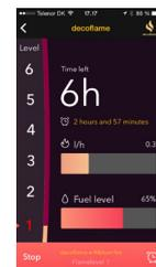
6. For adjusting the flame intensity, select the desired level on the left side of the screen. (1-lowest and depending on model 5-highest + Eco-Wave or 6-highest). Should there not be enough fuel for the selected burning time - the fireplace will shut down automatically. Select 'STOP' to turn off the fireplace.
