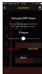
5. For the 'Turn Off Timer' press the clock icon in the lower right corner. To adjust the remaining time, slide the dot to the left and right and select 'SET TIMER'.
